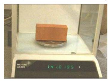
On a top loading laboratory balance (this one reads to  $0.0001\,\mathrm{g}$ ) a  $140\,\mathrm{g}$  sample of reheated brick will gain mass at a fast enough rate to see the last digit increase as you watch.
